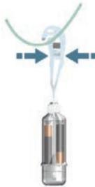
1. Place snap into the groove in the locking collar
